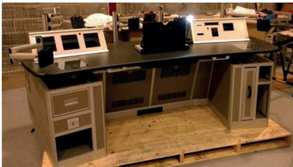
Thinking Space are currently in the process of supplying seventeen consoles bound for Abu Dhabi. The brand new air traffic furniture, which has electrical height adjustment, has been custom designed to fit within ATC towers and for ATC simulators at various sites.
